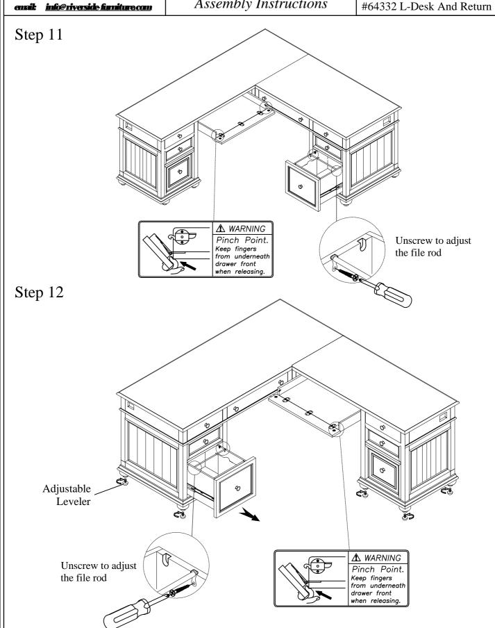
The levelers in the bottom of the Bun Feet can be adjusted if necessary to compensate for uneven flooring
